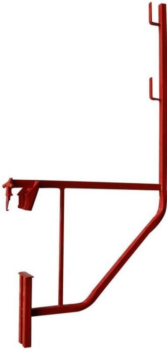
This picture is a side view of a scaffold bracket. This bracket is mounted to the stud and can be hung over a top plate. Two 2 x 10's are placed on the flat section to create a 18 inch walking surface. 2 x 4's are installed on at the vertical uprights to create a top rail and mid rail.
